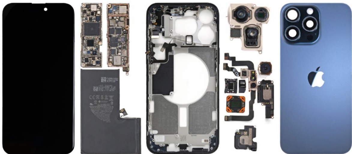
Figure 5.i. A ‘teardown’ image showing the major component blocks of an iPhone 15 Pro Max.
