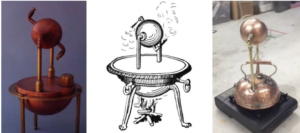
Figure 3.x. The aeolipyle: (left) a model at rest; (centre) a drawing; and (right) a model in use — the nozzles are blurred due to the speed of rotation 173 .
